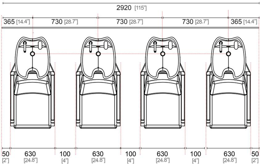
If washing from side add 400mm between each basin. All measurements in mm.
